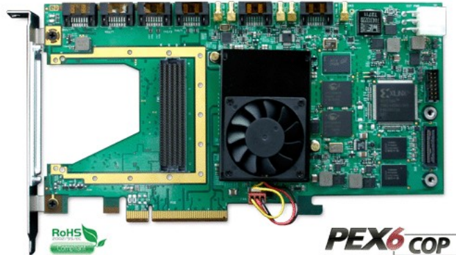
(BGA cooler obscures FPGA)
